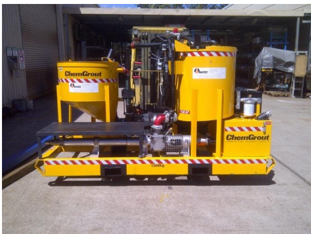
Blackrock Mining's custom built grouting system
